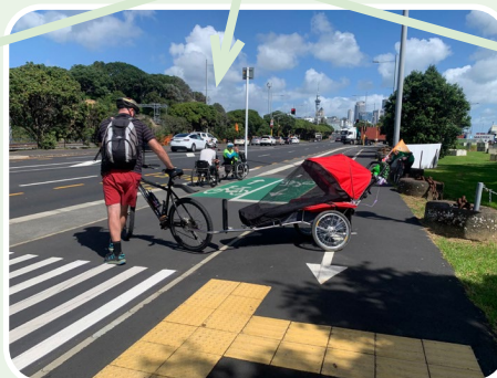
Here the trailer bike had to turn around, which resulted in blocking the entire cycleway and footpath
